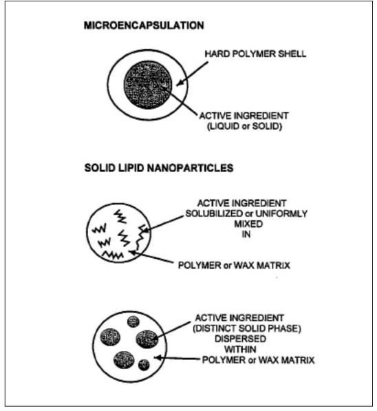
Figure 17.1. Schematic comparing microcapsules with SLNs.
