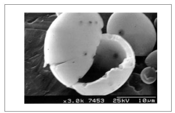
Figure 17.3. SEM of fractured poly(4-vinylpyridine) microcapsule.
