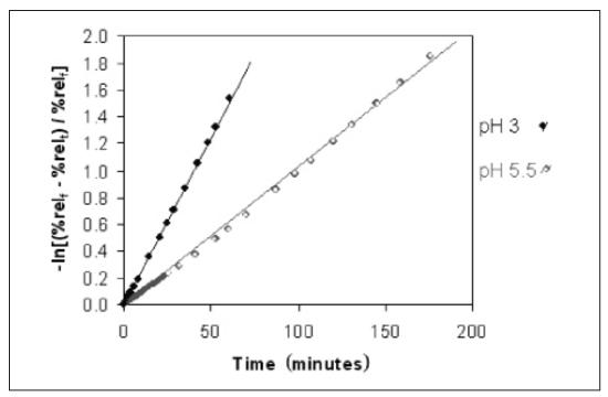
Figure 17.4. pH dependent release kinetics from a PVPy microcapsule
