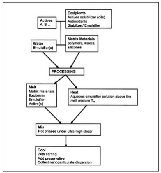
Figure 17.5. Schematic of the Melt-Emulsify-Chill process.
