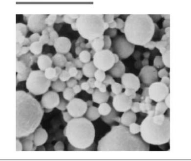
Figure 17.6. SEM of a typical SLN. Note that the particles are spherical but polydisperse.
